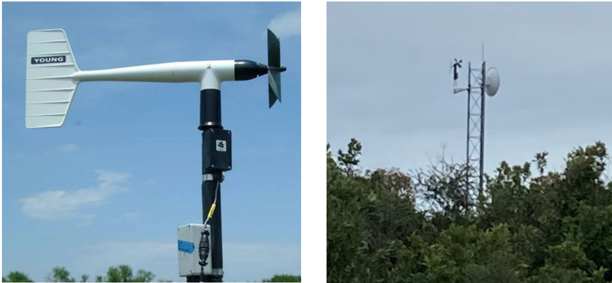
Figure 4 – Left: Marine-grade anemometer used at the BDCF. Right: Anemometer (and Ethernet antenna) mounted to the dune tower erected near the Shore Station (photo taken from A1A).
